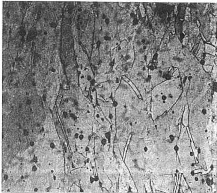
Figure 9 Flat section of Sarazm 6 (magnification, \times 256 ) showing the distortion clearly. Here it is seen that the recrystallization is not complete.
