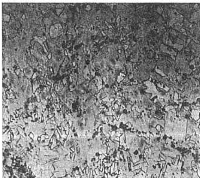
Figure 2 Sarazm 2 microstructure (magnification, \times 256 ) showing recrystallized grains with some distortion due to further hammering after annealing. Note the curved twins
