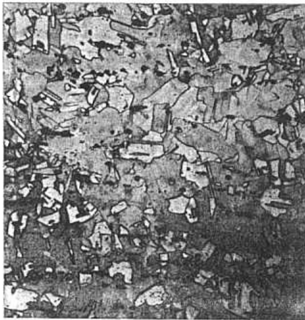
Figure 3 Sarazm 3 (magnification, \times 256 ) showing the islands of the recrystallized grains and the large pits which formerly held Pb, lead sulfide and lead sulfate particles.
