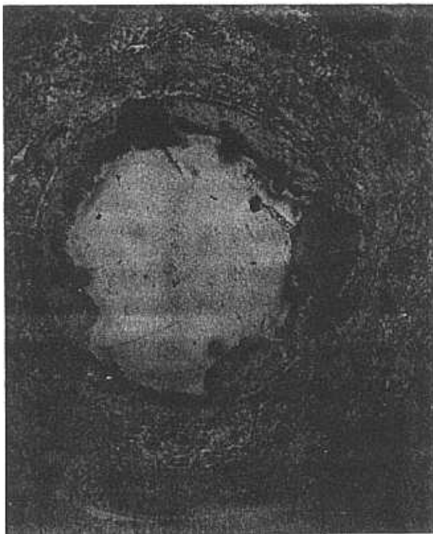
Figure 12 Sarazm 8 (magnification, \times 64 ). Cerargyrite bead showing a sharply cut hole.
